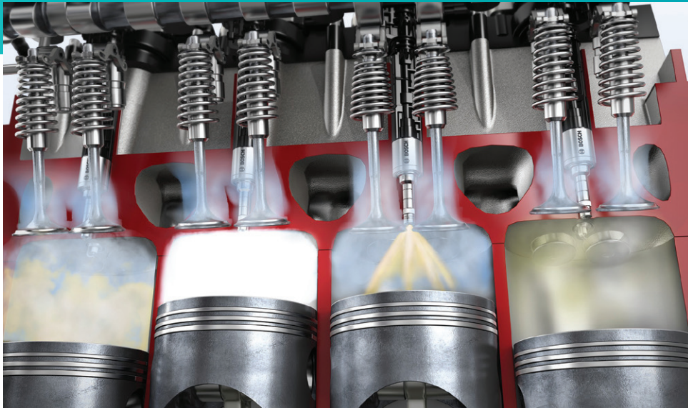
Bosch gasoline direct injection helps reduce fuel consumption by up to 15 percent while enhancing driving enjoyment.
