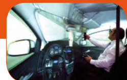
Stereoscopic multiple walls immersive visualization system used in the ergonomic assessment of a car cockpit
