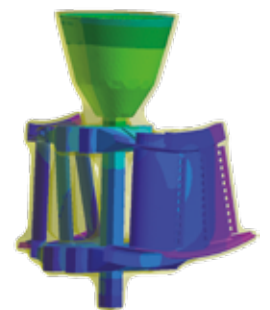
NGV Blade with Realistic Shell Modelling
