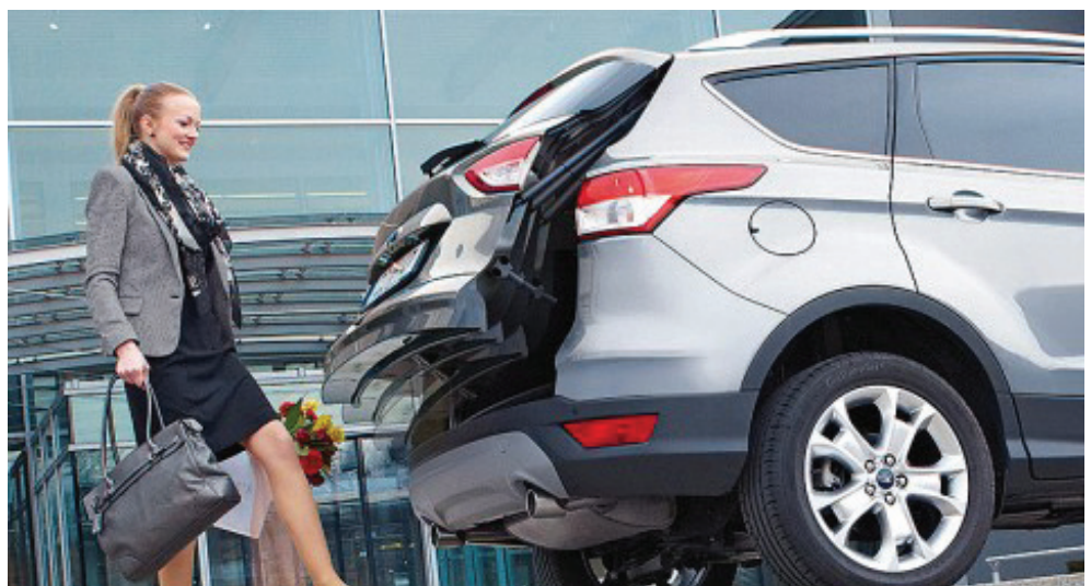
The patented Brose system for contactless opening and closing of luggage compartment doors represents a new level of comfort for vehicle access.
