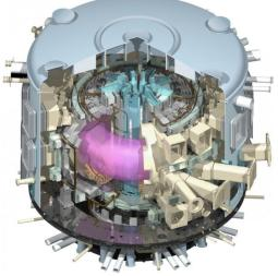
In comparison to nuclear power plants, the tokamak structure itself also provides benefits in terms of safety. The tokamak cannot explode and does not leak or have poisonous, dangerous by-products. It can be safely shut down if an accident occurs, as long as the heat of the system is contained.
